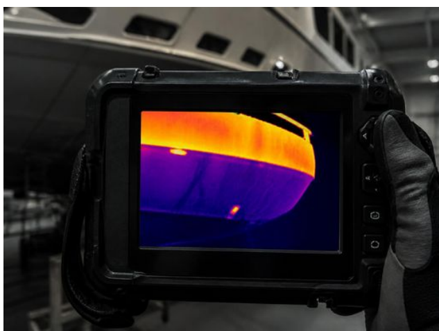
THERMAL IMAGING AND MOISTURE MAPPING
